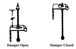
Figure 7. Adjust Damper Cable
