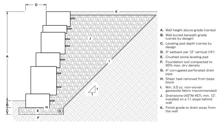
This page shows typical construction details for Outcropping walls. These drawings are representative of major components required in wall construction. Specific details including geotextile reinforcement layers, drainage details, soil requirements, etc. shall be per engineered design for wall. For more cross-section and design options, visit our website.
