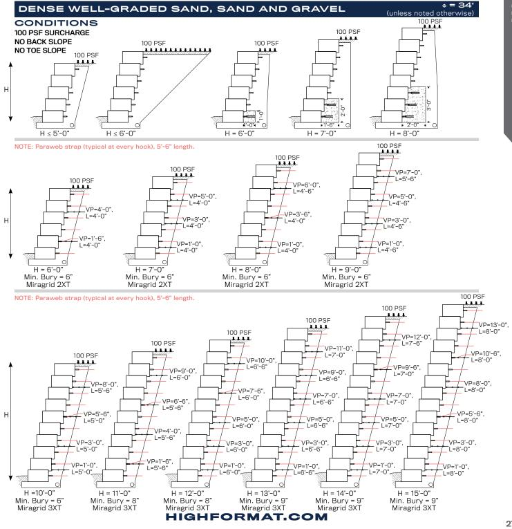
This page shows preliminary guides for soil reinforcement required to construct a wall with HIGH FORMAT® Outcropping blocks in the conditions noted below. Refer to typical wall sections for all other details.
