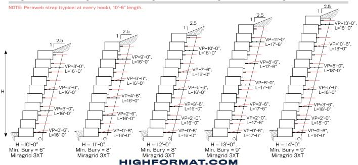
This page shows preliminary guides for soil reinforcement required to construct a wall with HIGH FORMAT® Outcropping blocks in the conditions noted below. Refer to typical wall sections for all other details.
