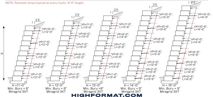
This page shows preliminary guides for soil reinforcement required to construct a wall with HIGH FORMAT® Outcropping blocks in the conditions noted below. Refer to typical wall sections for all other details.
