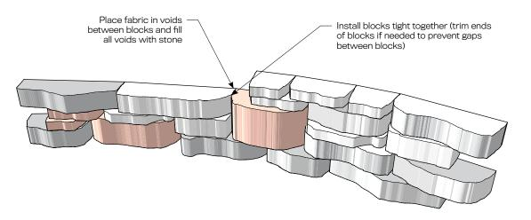
This page shows typical construction details for Outcropping walls. These drawings are representative of major components required in wall construction. Specific details including geotextile reinforcement layers, drainage details, soil requirements, etc. shall be per engineered design for wall. For more cross-section and design options, visit our website.
