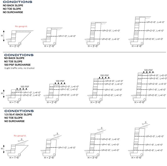
This page shows preliminary guides for soil reinforcement required to construct a wall with HIGH FORMAT® Belvedere® wall blocks in the conditions noted below. The geogrid reinforcement is Mirafi Miragrid 2XT. The geogrid layers shall be placed with 100% coverage along the length of the wall (no gaps between sections of grid). Refer to typical wall sections for all other details.
