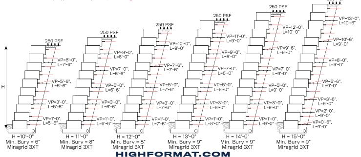
This page shows preliminary guides for soil reinforcement required to construct a wall with HIGH FORMAT® Outcropping blocks in the conditions noted below. Refer to typical wall sections for all other details.
