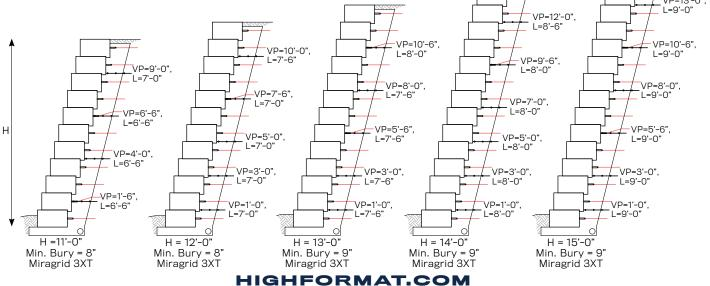
This page shows preliminary guides for soil reinforcement required to construct a wall with HIGH FORMAT® Outcropping blocks in the conditions noted below. Refer to typical wall sections for all other details.
