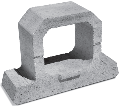
Premier 6's bottom-side anchor bar creates an automatic 4.7° setback.
