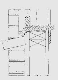
Flat sawed-stone sills may be tipped for wash surface, or set flat in windows or as capping for wing-wall extensions. This is particularly effective when used as band course at sill level. Dealer or his supplier can provide specially sawed shapes where checked-out areas are needed.
