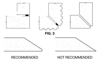
For economy, design rustication only on one side of a joint. (See Fig. 4.)  If exposed stone patios occur over a heated room, insulate the ceiling of the room. Warm stones absorb moisture, and a sudden drop in outside air temperature may freeze and crack the stone. (See p. 31 and 63 for recommendations on large horizontal areas.)
