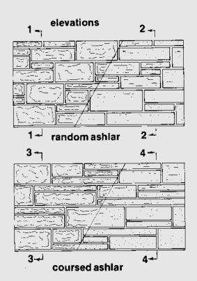
Random ashlar and coursed ashlar are both made from strips of limestone with lengths cut as desired at the jobsite. The only real difference between them is that the mason lays to a line with one (coursed) and does not with the other (random).
