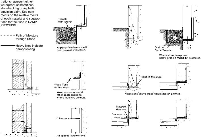
**Note:** Isolate stone from grade moisture with a concrete ledge or a dampproofed starter course with flashing as shown.
