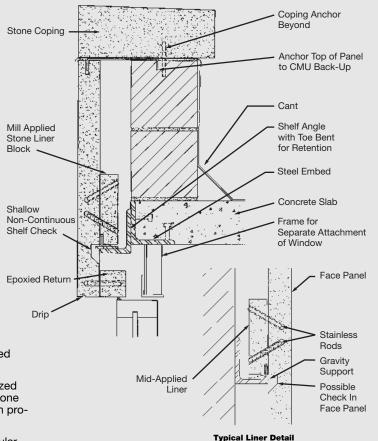
Also designs should be avoided that might transfer unintended and unplanned loads into panels and the liners through connection points, hard joints or other paths.
