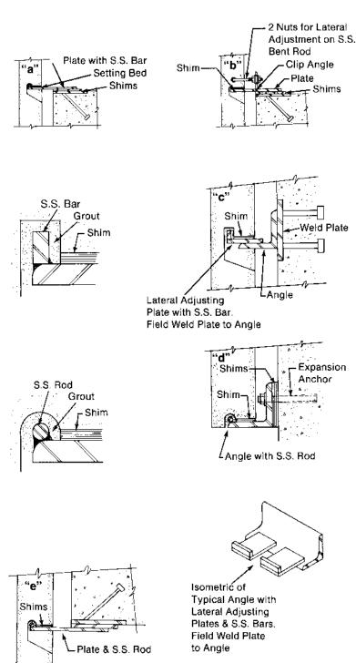
Angle with S.S. Rod S.S. Side Anchor Adjustable Shim Concrete Insert with Askew Bolt, Nut & Washer Shim Angle Steel Shims Weld Plate Shim Angle with S.S. Rod Shim Weld Plate Angle Lateral Adjusting Plate with S.S. Bar. Field Weld Plate to Angle
