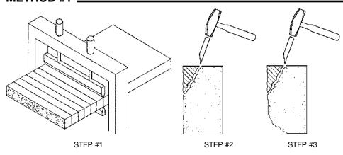
STEP #1—A stone slab is guillotined or broken into individual pieces by a machine.
