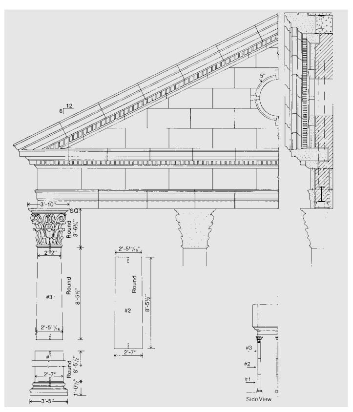
Column drum beds, and the beds of column bases and capitals, should be matched to their membering surfaces in the mill prior to shipment. The stone fabricator has the responsibility to produce column parts to the tolerance allowed for other "critical depth" situations.
