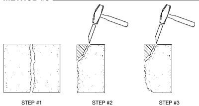
STEP #1—A sawed-6-sides stone slab is drilled and split to obtain two pieces of rock face.
