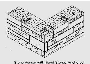
to Concrete Block Backing.
