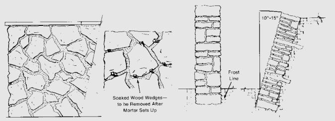
Webwall patterns are attractive and easy to set. The webwall style is a veneer and must be set against a firm backup and on a solid foundation or ledge. Shaping stones with mallet or chisel can create smaller joints. Wedges may be used occasionally to hold stones in place until mortar sets. Sawed wall coping is particularly effective used with these freeform patterns.
