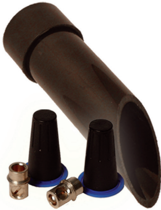
CS100 Buried connection point for central point (spider) wiring. Includes two brass connectors with set screws and plastic lug caps in PVC housing. When installed: 2.5" diameter x 9.15" depth.
