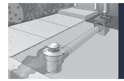
The Pop-up Drainage Emitter is an easy, safe and efficient solution that allows water to be diverted and released to water-safe areas away from structures, erosion-prone landscapes and poor drainage areas.
