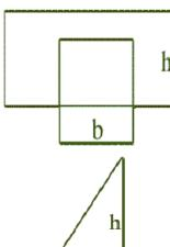
Area of a Triangle = (Width x Height) divided by 2 Example: "b"ase is 8 feet and the "h"eight is 12 feet 8'x12'= 96, then divide by 2 = 48 sq ft (resulting in 5 rolls)
